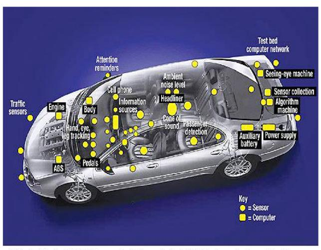
1. Daimler-Chrysler's 300M IT concept vehicle embodies the fully instrumented car of the future. It uses a variety of sensors to help drivers concentrate on the road for safer driving.
