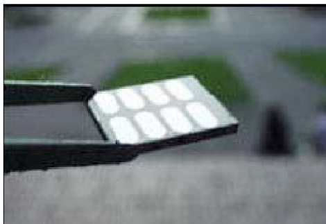
Figure 3: Schematic diagram of a hybrid "plastic" solar cell with a nanorod/polymer layer sandwiched between two electrodes. The middle layer, a mere 200 nanometers thick, is a jumble of nanorods embedded in the semi-conducting polymer.
