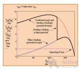
The above figure represents the torque vs speed characteristics of a single-phase induction motor.
